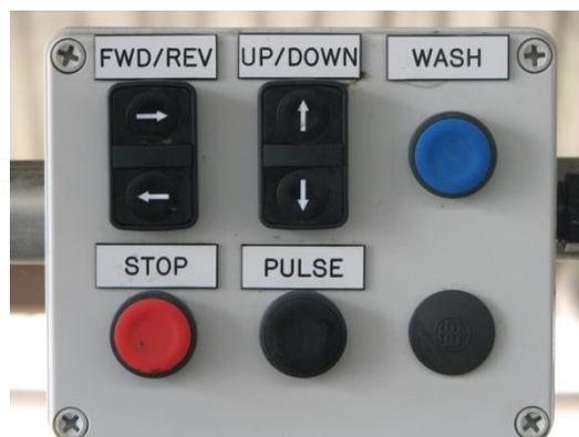
**To raise gate:** push up button, gate will rise to up position if no stop is pushed.
