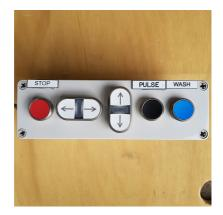
To raise gate: push up button, gate will rise to up position if no stop is pushed.
