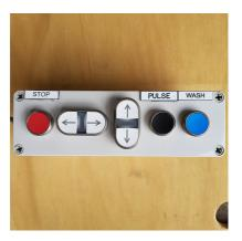
To raise gate: push up button, gate will rise to up position if no stop is pushed.
